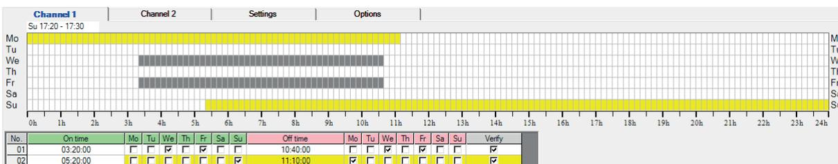
Figure 23: Switching ON and OFF on different switch-on and switch-off days (yellow marked)
