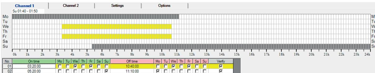
Figure 72: Switching ON and OFF on the same switch-on and switch-off days (yellow marked)
