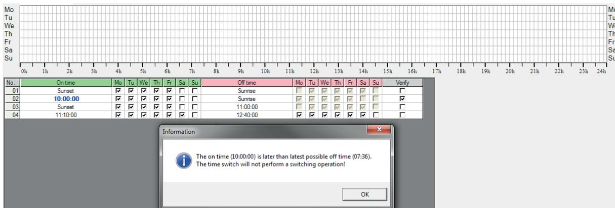
Figure 91: Warning message: Switching-off at sunrise, the switching-on time lies after the latest possible switching-off time
